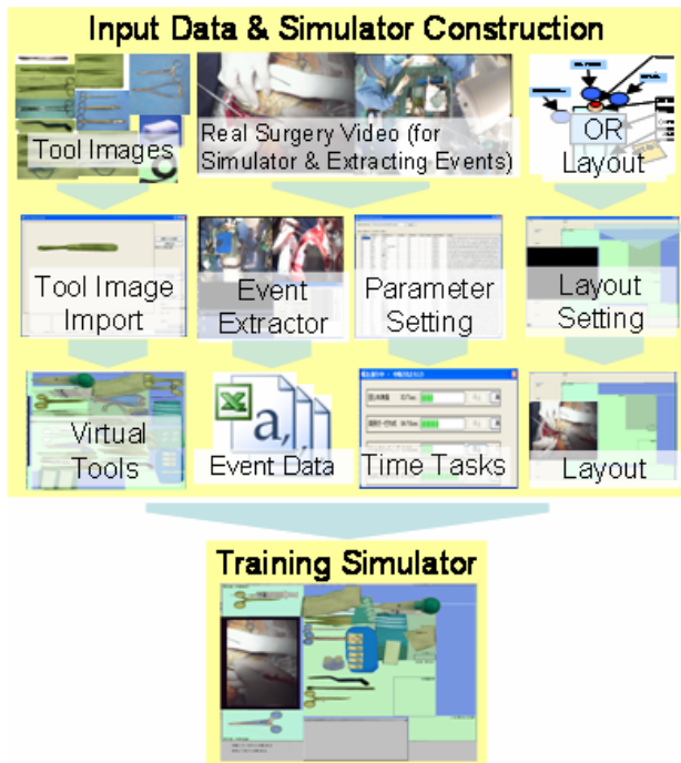
Fig. 11 Construction of training simulator
